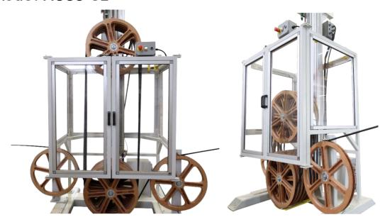
The DRTS accumulator is designed to provide a time buffer during the pipe production useful when beginning a new coil. Accumulation is vertical to minimize floor space. The upper rollers move vertically while the bottom rollers are fixed. All rollers are idle (non-driven) and are designed specifically for drip irrigation as well as plain pipe of varying diameters. The accumulator is automatically synchronized to the production line.
