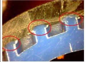
Melt temperature can be controlled at the Crosshead zone. Too high and the labyrinth is melted. Too low and the bonding is incomplete.
