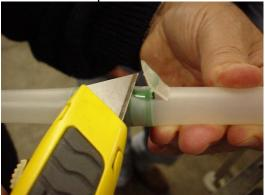
Make sure that the Perforator drilling of the pipe is not scratching the dripper pool. Even minor scratch marks indicate the occasional possibility for small punctures in the dripper which greatly increas flow.
