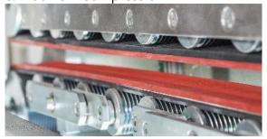
Make sure the hauloff/puller of the pipe does not smash the drippers. It should be adjusted to a minimum that consistently pulls the pipe. V grooved belt on the haul-off is recommended. Too much compression on the drippers from the Haul-Off can cause low flow and inconsistency. DRTS uses a unique hauloff design that regulated the pressure with air as well as use a floating belt mechanism to reduce the pressure on the dripline.
