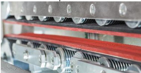
Make sure the haul-off/puller of the pipe does not smash the drippers. It should be adjusted to a minimum that consistently pulls the pipe. V grooved belt on the haul-off is recommended.
