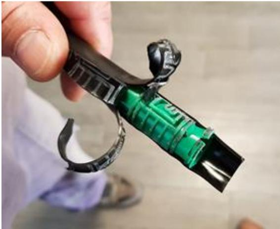
Melt temperature can be controlled at the Crosshead zone. Too high and the labyrinth is melted. Too low and the bonding is incomplete.
