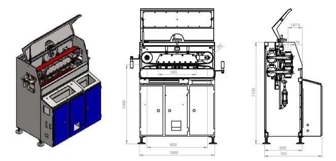
The DRTS Servo Haul-off can be easily installed on existing lines without making any changes. Communication with existing extruders can be made using any protocol. The puller is specifically designed for drip pipe or plain pipe of varying diameters. Due to the special design, the pulling speed is very stable despite the normal issues associated with drippers in the pipe.
