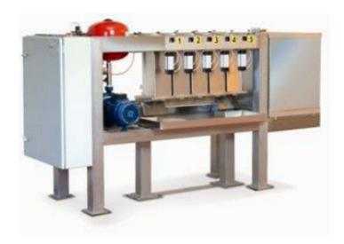
The DRTS Flow Tester can test any type of emitting device from drip tubing and drip tape to button drippers and sprinklers. Using load cells to measure the collected water allows a very high accuracy of flow measurement in the shortest possible time as samples are tested simultaneously.
