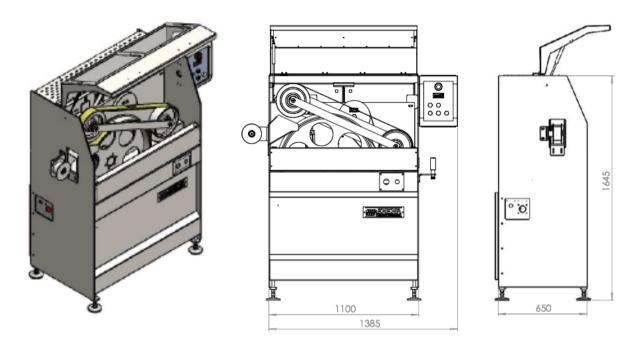
The DRTS Capstan Haul-off can be easily installed on existing lines without making any changes. This high speed Haul-off unit is intended for thin-wall pipe. This unit requires almost no maintenance and has very low wear of parts (no belts). The use of only one motor makes it very energy saving. As no belts are use, there is no friction, making the operating speed very stable.
