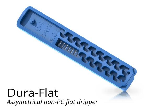
This compact emitter for agriculture features a wide flowpath cross-section and extra large filtration area for effective, efficient performance and excellent clogging resistance.
