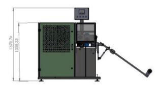
The DRTS Re-coiler is designed to give manufacturers the ability to re-coil unfinished coils or create short coils from a larger coil. This machine reduces your scrap rates by allowing you to utilize the good sections of a produced coil which would normally be scrapped.
