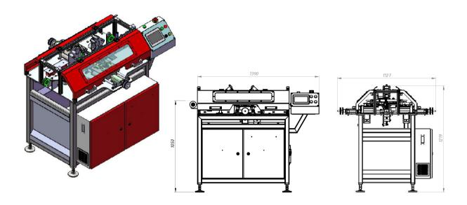
The DRTS Servo Perforator can be easily installed on any existing line without making any changes. It has its own line speed encoder making it an autonomous machine. Spacing measurement including historical report can be retrieved directly from the PLC or via USB port. Hole position can be adjusted via the touchscreen at a resolution of  $\pm$ 0.01mm. The depth of the hole can also be adjusted during operation at a resolution of  $\pm$ 7-0.1mm.
